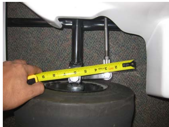
Correct Spindle length. Close to the edge of the wheel rim
