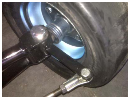
Incorrect Spindle Arm length, tie rod end rubbing on tire.
